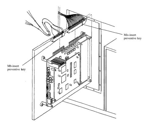
3 Put the PC board installed on the install board into the cabinet
