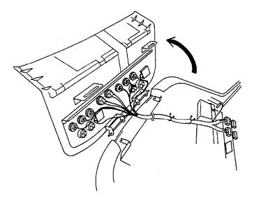
3 If the control panel of your cabinet is different from the above drawing, refer to the operation manual of your cabinet and replace the control panel or add/reduce button switches. If some switches are reduced, be sure to fill up the switch holes with hole caps. 4 Connect the wires of the extended edge harness on the following table to the terminals of PI button switch 4,5,6 and P2 button switch 4,5,6 on the control panel by soldering or fixing an applicable crimp-style terminal.
