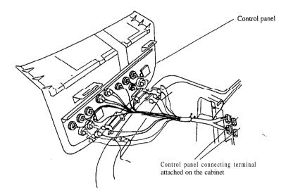
• In case the button switch is three-terminal, the input terminal (such as **1P\_PUSH1**) of the control panel connecting terminal should be connected to the N.O. terminal of the button switch. GND of the control panel connecting terminal should be connected to the COM terminal of the button switch.
