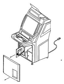
3 Disconnect the cables and harnesses connecting to the PC board.
