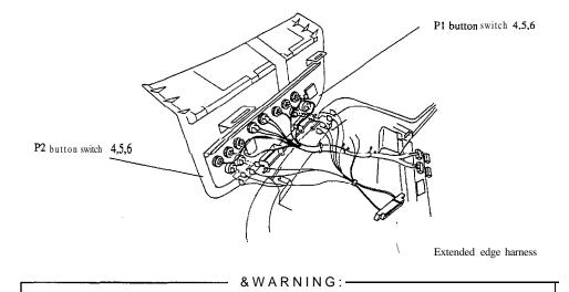
Always use the extended edge harnes specified by Namco Ltd. Otherwise it may cause a fire or electrical shock. Contact your distributor to order parts. Refer to "11. REPLACEMENTPARTS LIST," on pp.56foordetails of the regulacement parts.
