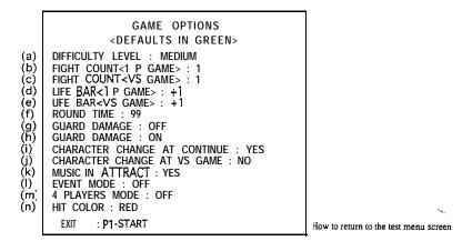
Hit the Pl S-direction joystick up or down to select an item to change the setting out of (a) • (i) on the above figure. The selected item is highlighted in red.
