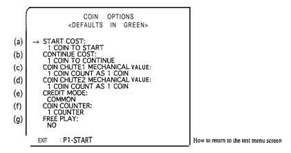
2 Hit the Pl S-direction joystick up or down to select an item to change the setting out of(a) • (g) on the above figure. The selected item is highlighted in red.
